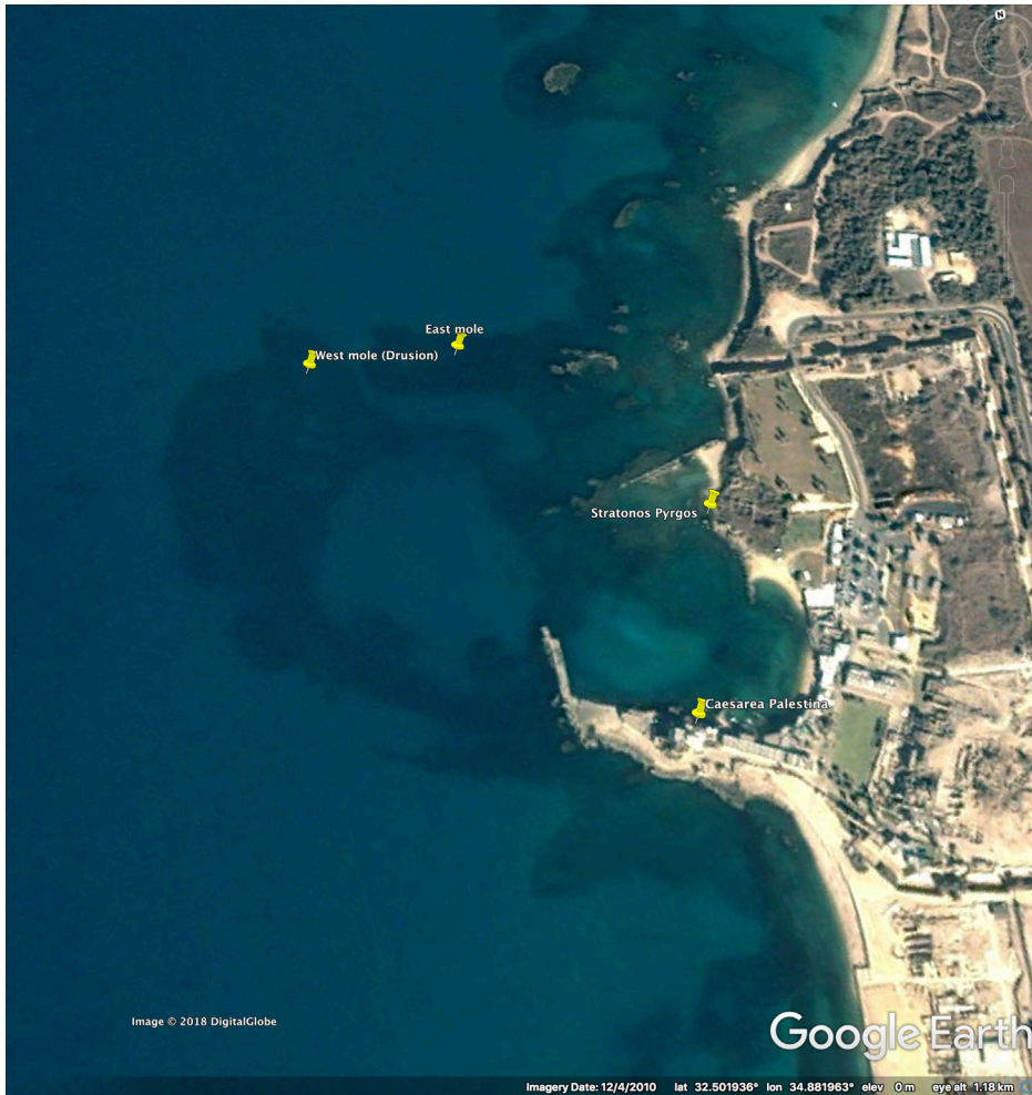
Fig. 6-37: Aerial view of the harbour at Caesarea Palaestinae (Sebastos), built by King Herod 22 to 10 BCE. 85 An inner and outer port are clearly visible underwater. The port entrance was on the more sheltered northerly direction and it is on either side of this entrance - labelled east and west moles - that towers are thought to have been constructed. Two towers may have stood just outside the entrance, bearing statues of Meriamme, Herod's favourite wife, and of Phasael, a dead brother. Hippius, a friend killed in battle was the dedication for a third, larger tower that was built on the end of the east mole, on the port side of the entrance. On the starboard side (west mole) of the entrance, where there is the greatest concentration of underwater debris, it is commonly accepted as being the site for a grand lighthouse on the same design but smaller in scale, as the Alexandrian Pharos. This lighthouse was known as the Drusion tower. The lengths of the moles were punctuated with minor fortifications at regular intervals. Another lighthouse tower in the inner harbour cannot be ruled out.
