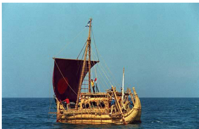
Fig. 2-7: Ra II, a reconstruction of the kind of papyrus reed boat suitable for long-distance sea crossings, as proposed by Thor Heyerdahl in 1970. 63
