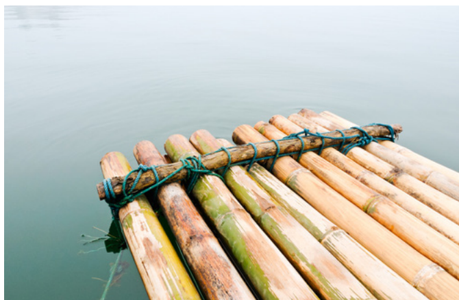
Fig. 2-5: A primitive raft showing ten straight logs, each capable of carrying a single human, bound together into a raft. In principle, no metals tools are necessary. 63
