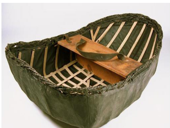
Fig. 2-9: A skin-covered wooden framed boat known as a coracle used by Celtic peoples of north-west Europe. Similar boats are also found in India, Viet Nam and Tibet. 66
