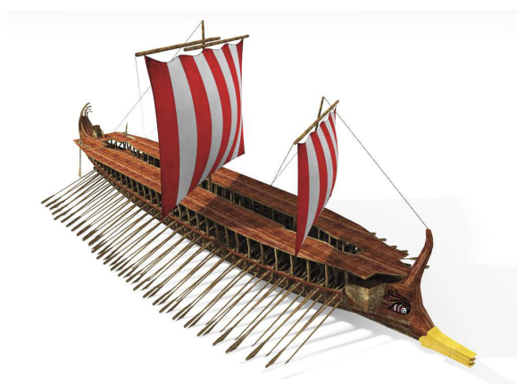
Fig. 2-14: Model of an Egyptian trireme powered by both oars and sails (square rigged). 68
